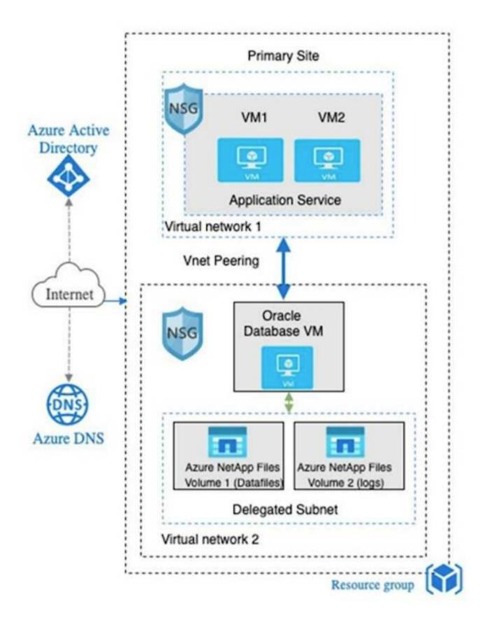
The Azure Oracle environment can be managed with an Ansible controller node for automation using tool kits provided by NetApp for database deployment, backup, recovery, and database migration. Any updates to the Oracle Azure VM instance operating-system kernel or Oracle patching can be performed in parallel to keep the primary and standby in sync. In fact, the initial toolkits can be easily expanded to perform daily Oracle tasks if
