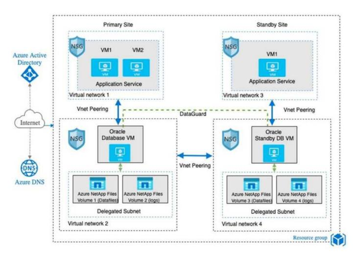
In many respects, the implementation of Azure NetApp Files in Azure cloud is very similar to an on-premises ONTAP data storage architecture with many built-in redundancies, such as RAID and dual controllers. For disaster recovery, a standby site can be setup in different regions and database can be synced up with the primary site using application-level replication (for example, Oracle Data Guard).
