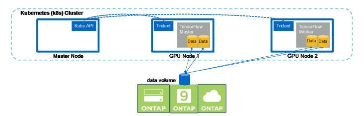
1. The following example commands show the creation of one worker that participates in the synchronous distributed execution of the same TensorFlow benchmark job that was executed on a single node in the example in the section Execute a Single-Node Al Workload. In this specific example, only a single worker is deployed because the job is executed across two worker nodes.
