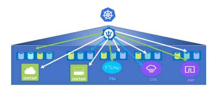
ONTAP Storage Virtual Machine (SVM) provides secure multi-tenancy. A Single OpenShift cluster can connect to single SVM or multiple SVMs or even to multiple ONTAP clusters. Storage class filters the backend storage based on parameters or by labels. Storage administrators define the parameters to connect to storage system using trident backend configuration. On successful connection establishment, it creates the trident backend and populates the information which the storage class can filter.
