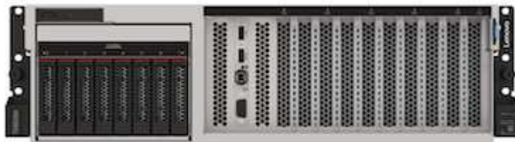
4x double-wide or 8x single-wide GPU slots and 2x PCIe I/O slots with 8x 2.5-inch or 4x 3.5-inch HS drives
