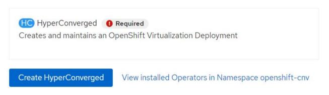
8. On the Create HyperConverged screen, click Create, accepting all default parameters. This step starts the installation of OpenShift Virtualization.
