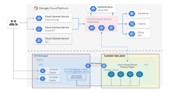
The part above the dotted line shows the control plane of the service, which controls the volume lifecycle. The part below the dotted line shows the data plane. The left blue box depicts the user VPC (service consumer), the right blue box is the service producer provided by NetApp. Both are connected through VPC peering.
