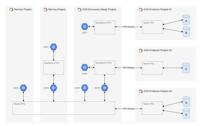
The preceding figure shows a project (the CVS consumer project in the middle) with three VPC networks connected to Cloud Volumes Service and multiple Compute Engine VMs (GCE1-7) sharing volumes:
