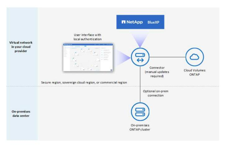
Meanwhile, the second image shows an example of a private mode deployment where the Connector is installed on premises, manages an on-premises ONTAP cluster, and provides access to supported BlueXP data services.
