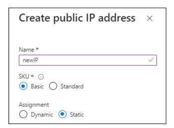
If you use a Standard SKU IP address instead, then BlueXP uses the *private* IP address of the Connector, instead of the public IP. If the machine that you're using to access the BlueXP Console doesn't have access to that private IP address, then actions from the BlueXP Console will fail.
