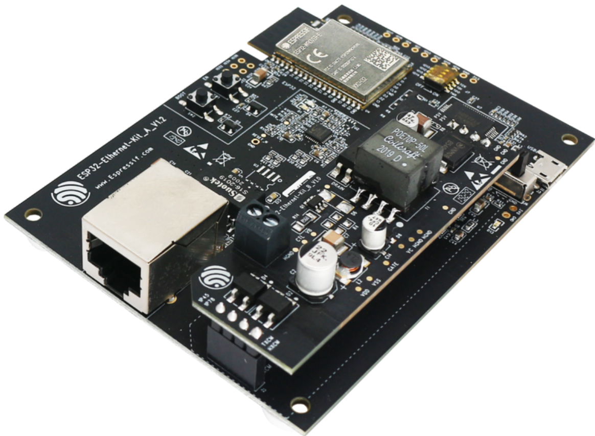
Fig. 20: ESP32-Ethernet-Kit V1.2 Overview (click to enlarge)
