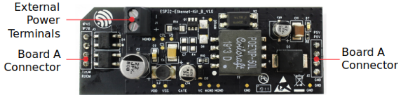
Fig. 34: ESP32-Ethernet-Kit - PoE board (B) layout (click to enlarge)
