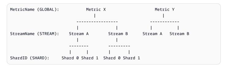
Not all metrics are available at the shard level; some are stream level or global by nature. These are not produced at the shard level, even if you have enabled shard-level metrics (Metric Y in the preceding diagram).
