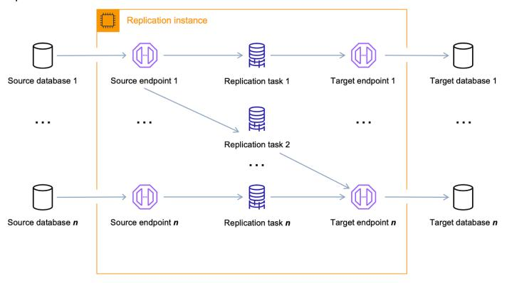
A single replication instance can host one or more replication tasks, depending on the characteristics of your migration and the capacity of the replication server. AWS DMS provides a variety of replication instances so you can choose the optimal configuration for your use case. For more information about the various classes of replication instances, see <a href="Choosing the right">Choosing the right</a> AWS DMS replication instance for your migration.
