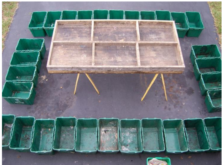
FIGURE 1: Layout of Hand-Sorting Table and Bins
