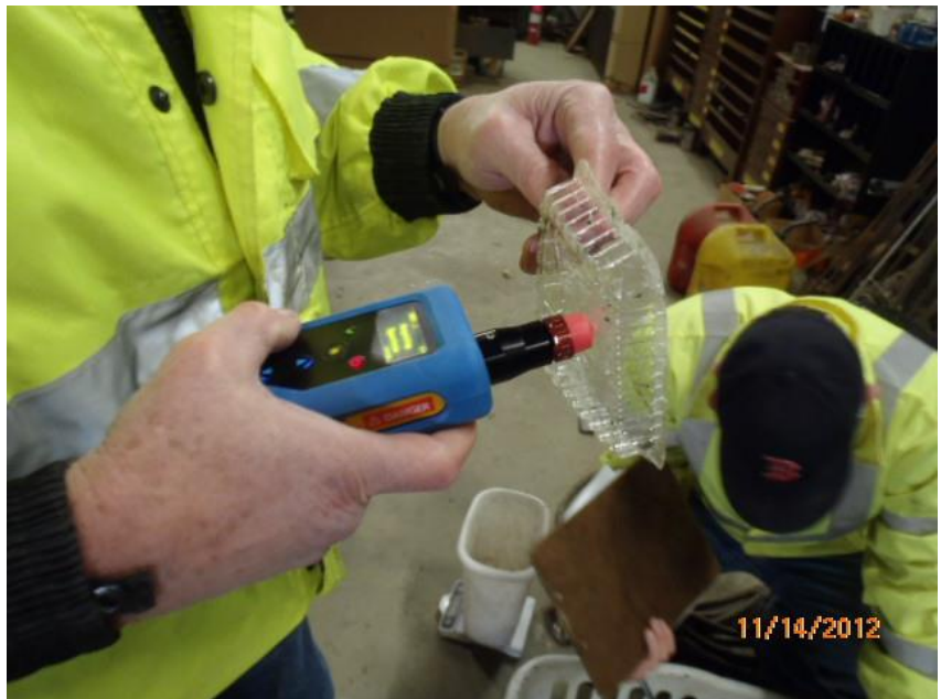
FIGURE 3: Delta Nu, V2 Plastic Resin Identification Meter
