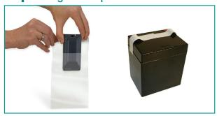
Place each required battery or cellphone in an appropriately sized bag. If no bags are available, cover the positive terminal with duct, and fold flap over. electrical or another non-conductive tape.
