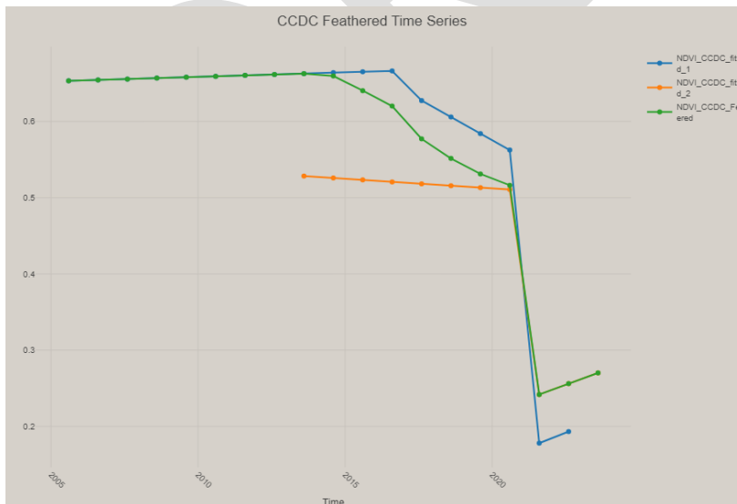
Figure 9. – An example time series showing the feathering of two CCDC image collections. The blue line is NDVI from v2022.8 CCDC collection, and the orange line is NDVI from v2023.9 CCDC collection. The green line is the weighted average of the two CCDC collections used in our models.
