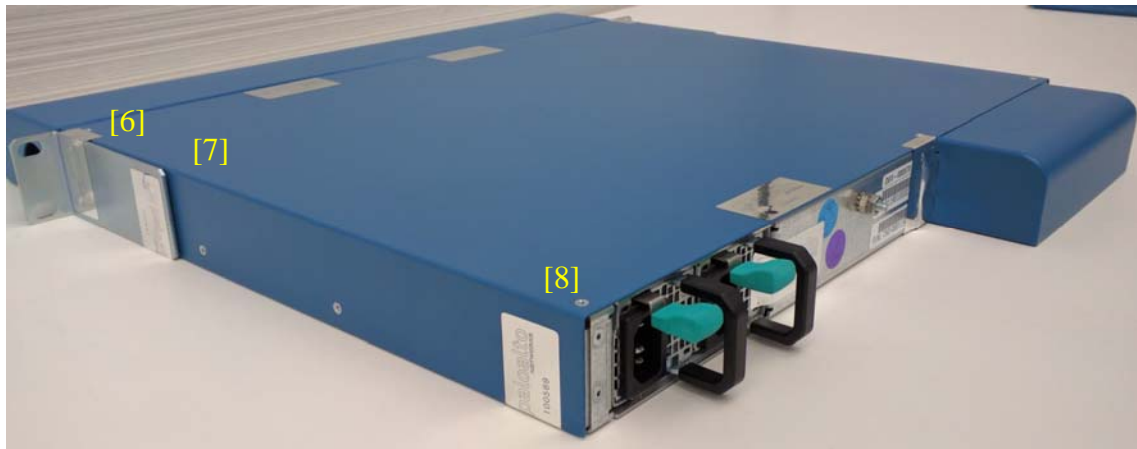
Figure 35 –PA-800 Right Side Rear Tamper Seal Placement (3)
