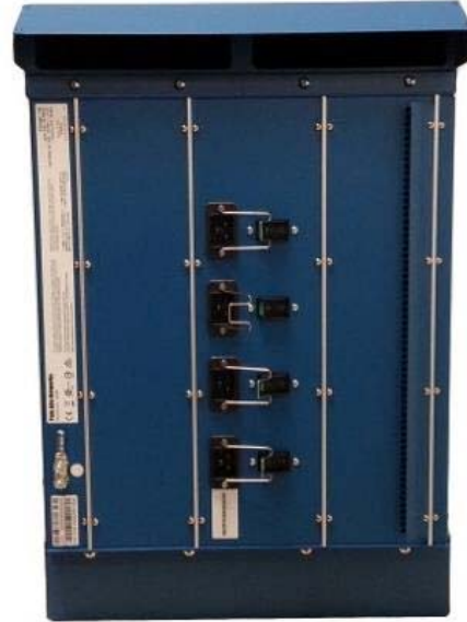
Figure 53 - PA-7050 Rear View with Opacity Shields
