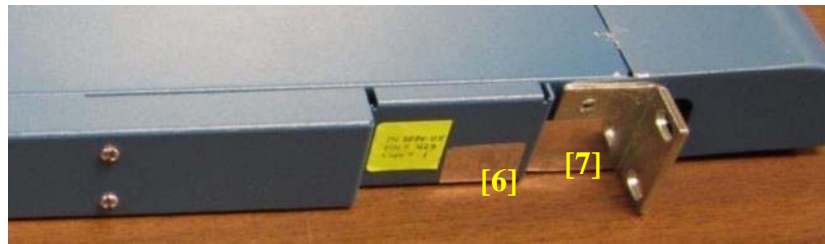
Figure 40 - PA-3020/PA-3050 Series Tamper Seal Placement (2)
