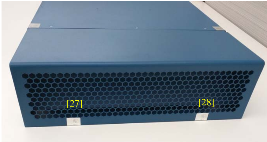
Figure 51 - PA-5200 Series Rear Opacity Shield
