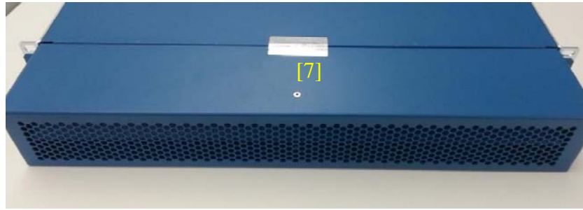
Figure 43 – PA-3060 Front/Top Tamper Seal Placement
