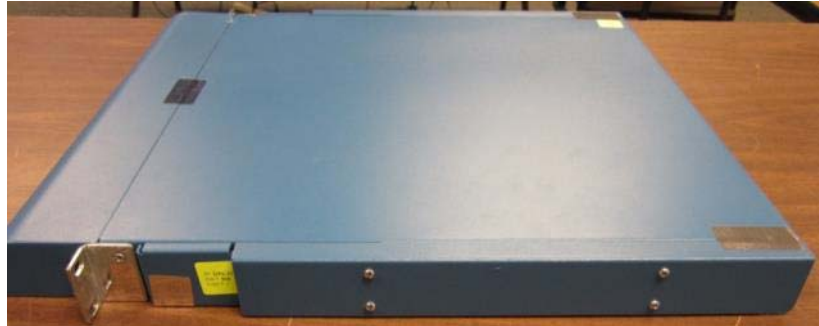
Figure 37 - PA-3020 / PA-3050 side with Opacity Shield
