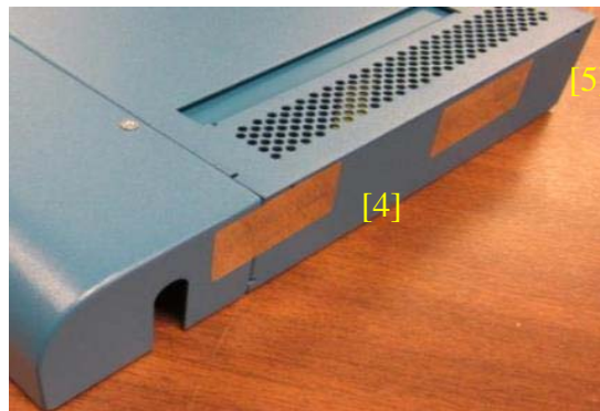
Figure 23 - PA-200 Right Side Tamper Seal Placement (2)
