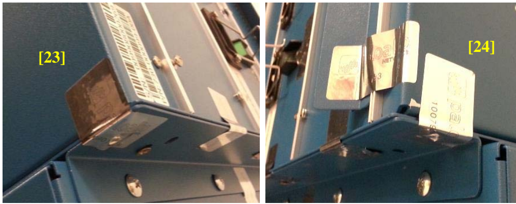
Figure 60 - PA-7050 Tamper Seal Placement for Bottom Plenum Bracket (23-24)
