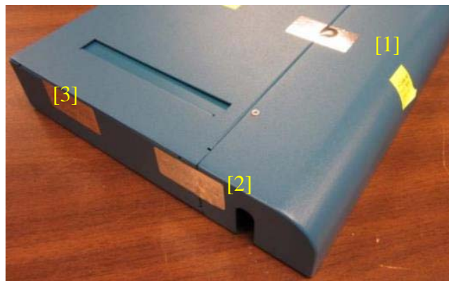
Figure 22 - PA-200 Left Side and Top Tamper Seal Placement (3)
