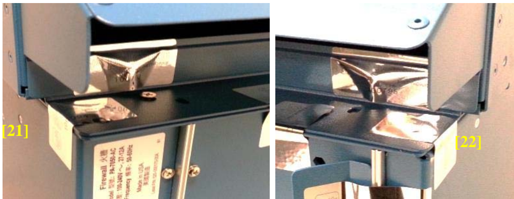
Figure 59 - PA-7050 Tamper Seal Placement for Top Plenum Bracket (21-22)
