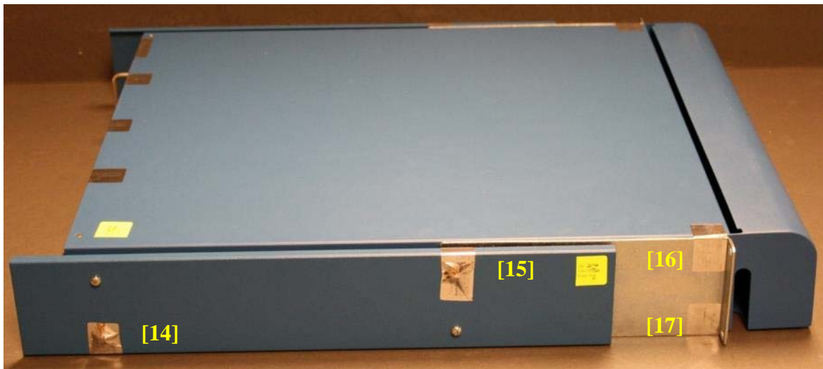
Figure 47 - PA-5000 Series Left Side Tamper Seal Placement (4)
