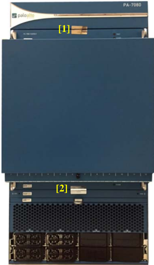
Figure 61 - PA-7080 Front with Opacity Shield
