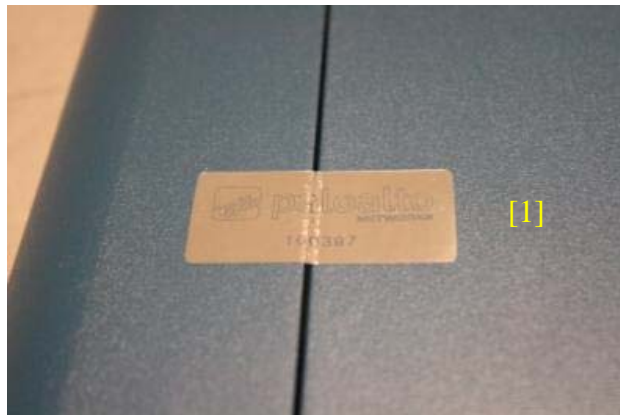
Figure 28 - PA-500 Front Tamper Seal Placement (1)
