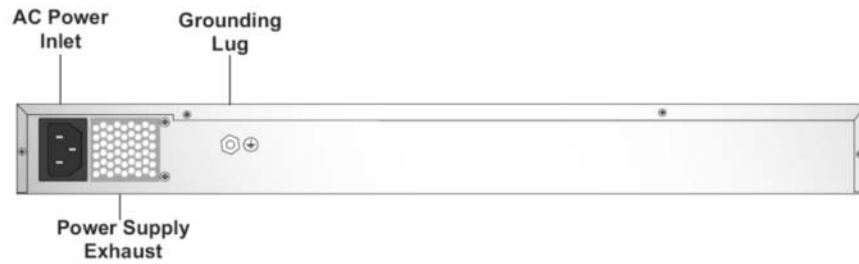
Figure 12 - PA-3020 / PA-3050 Back Interfaces
