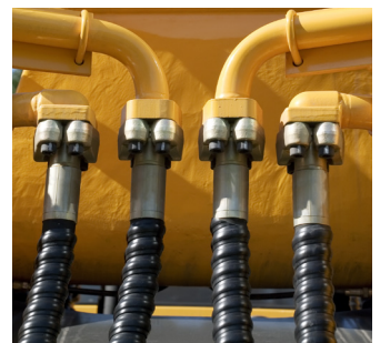
Typical High Pressure Hydraulic Lines
