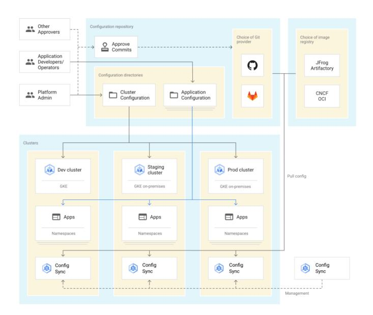
A Config Sync component per cluster pulls configuration directly from a source control repository or an image registry. A cloud management plane lets you centrally configure data sources and what tag or version of an application to pull. This cloud management plane means that you don't have to manually interact with each GKE cluster using the Kubernetes API to make individual config or application changes.
