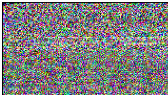
Fig. 3. A modulated CovertCast image for use in YouTube. Every colored block is 8 \times 8 pixels and encodes 6 bits of data.
