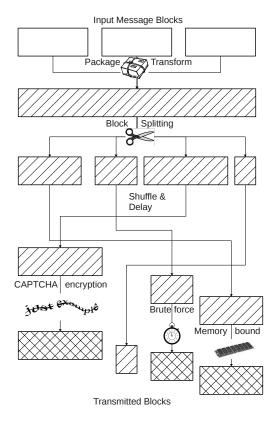
Fig. 1. Multi-stage scrambling of an input message. The package transform ensures that all steps must be undone to recover the original message.
