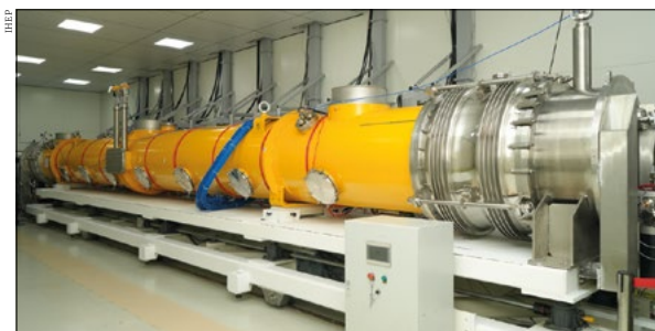
CEPC technologies A 1.3 GHz 8 × 9-cell cavity cryomodule (left) and a 650 MHz 800 kW continuous-wavelength, high-efficiency klystron (right) developed and tested at IHEP in Beijing.
