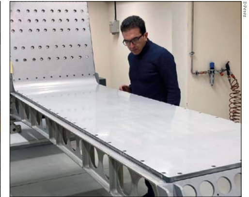
On schedule Vibration tests of a quarter of the new tracker layer taking place at INFN PG/SERMS Terni in Italy (left), and AMS chief engineer Corrado Gargiulo inspecting the prototype PDS radiator at CERN.
