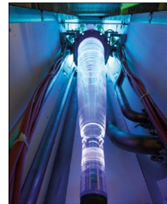
Enhancement A new quartz flow-tube system called FLOTUS was added to the CLOUD experiment in 2023 to allow pre-ageing of organic vapours before injection into the chamber.
