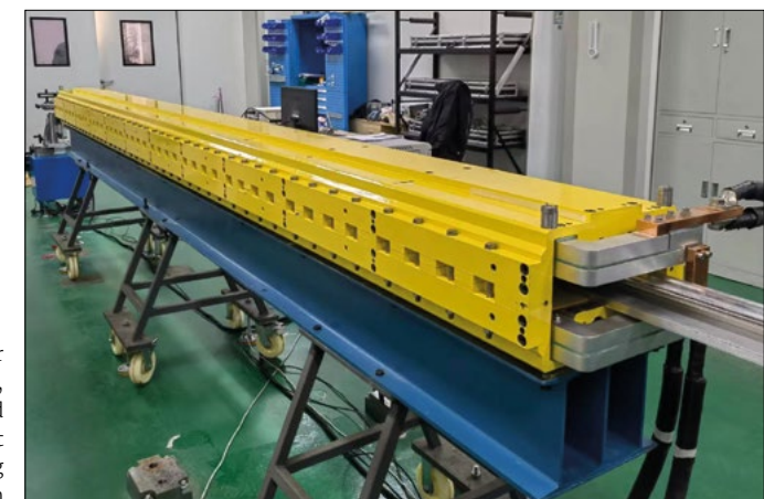
Boosting R&D A full-size prototype dipole magnet for the CEPC booster.
