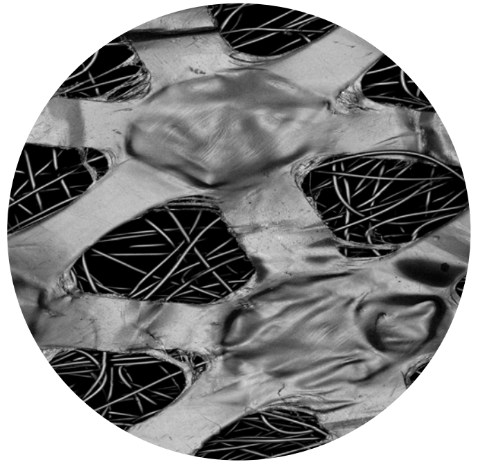
Band Aid pad viewed on the Olympus LEXT Optical Profiler
