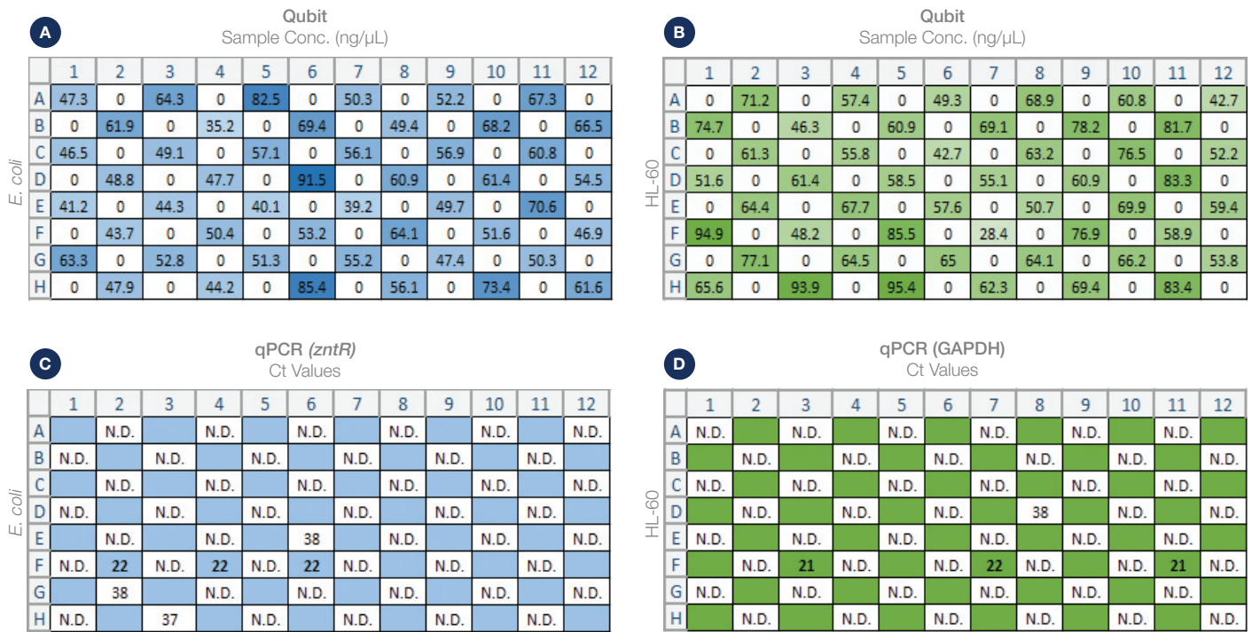
Figure 6: Qubit and qPCR assay of eluates to check for cross-contamination A&B); cross-contamination check by concentration measurements. White wells were filled with PBS. A) Blue fields were filled with bacteria and B) green fields were filled with human HL-60 cells resuspended in PBS. After the run, quantification was performed by using a Qubit system. Numbers indicate measured concentrations in ng/μL. C&D) To further increase the resolution of the cross-contamination check, three positive samples and all negative samples from the checkerboard runs were quantified by qPCR. Samples with cycle threshold values of \geq 35 or undetermined Ct value (N.D.) were considered negative.
