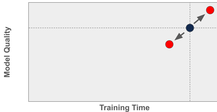
Figure 3: Applying a method to a model (red) could improve training time (x-axis) at the cost of model quality (y-axis), or improve model quality at the cost of training time compared to a baseline model (black). In either of these scenarios, determining whether the method constitutes an efficiency improvement requires examining a tradeoff curve (Figures 4 and 5).
