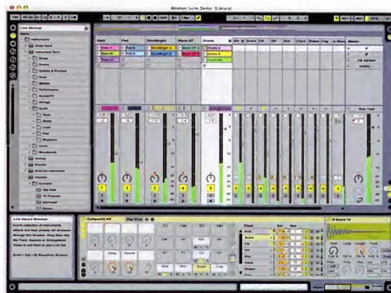
Many faces. This Live demo file shows the program's Browser pane (left), Session view (center), and Device pane (below).
