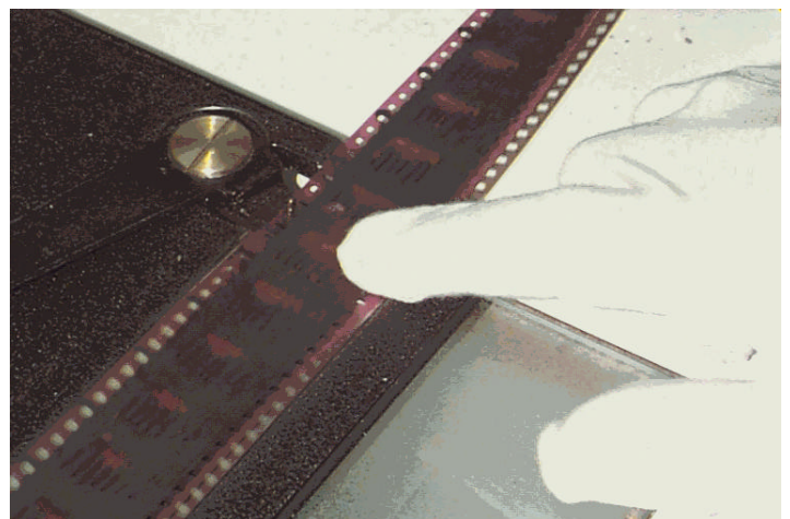
Figure 2: After counting the proper number of holes, slide the film over the pin attached to the pivoting arm.
