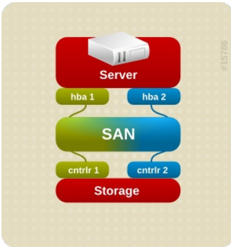
Figure 1.3. Active/Active Multipath Configuration with One RAID Device
