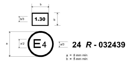
The above approval mark affixed to an engine/vehicle shows that, pursuant to Regulation No. 24, the engine/vehicle concerned has, with regard to the emission of visible pollutants by the engine, been approved in the Netherlands (E 4) under approval number 032439; the Regulation, at the time of approval, included already the 03 series of amendments. The corrected absorption coefficient is  $1.30~{\rm m}^{-1}$  (in the case of a vehicle approval).
