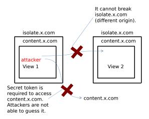
Figure 3. Isolating Views Using Pseudodomain Encapsulation
