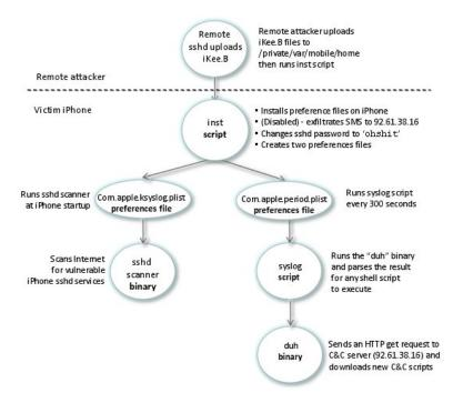
Fig. 1. Structural Overview of iKee.B
