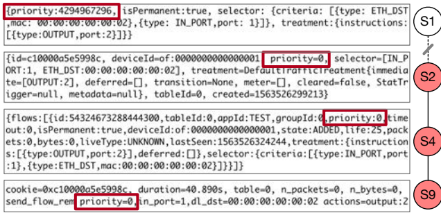
Fig. 9: Four different states of the flow rule based on the state diagram shown in Figure 8 of the ONOS controller.
