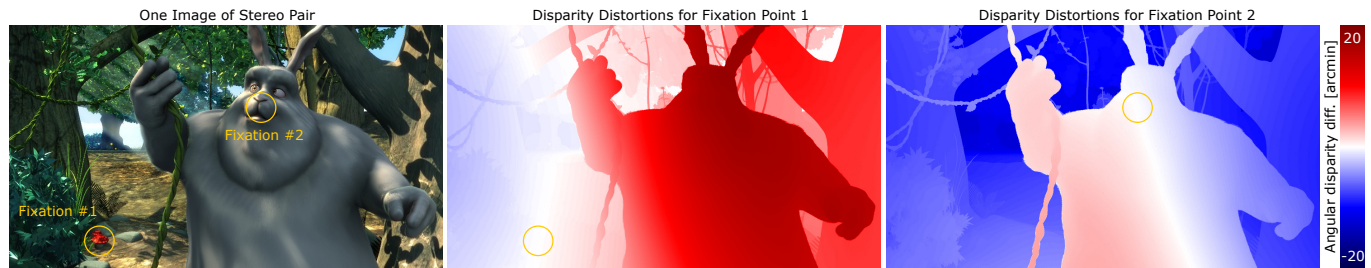
Fig. 1. Ocular motion associated with changes of fixation alters the positions of the no-parallax points in both eyes. Rendering models that do not account for ocular motion can create distortions of binocular disparity, as seen in this example. The color-coded error maps illustrate the magnitude of this effect as the difference between angular disparities resulting from classical and our gaze-contingent stereoscopic rendering for two different fixation points. Both shortening (red) and stretching (blue) of disparity gradients can be observed.
