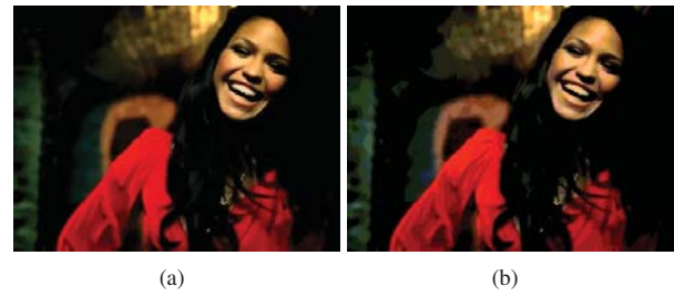
Fig. 5. (a) A frame from a testing animated GIF (3.221 bpp ); (b) The same frame after GIF optimization with threshold t = 0.125 (1.3222 bpp ). Although the storage gain is considerable, the quality loss can be visually perceived.
