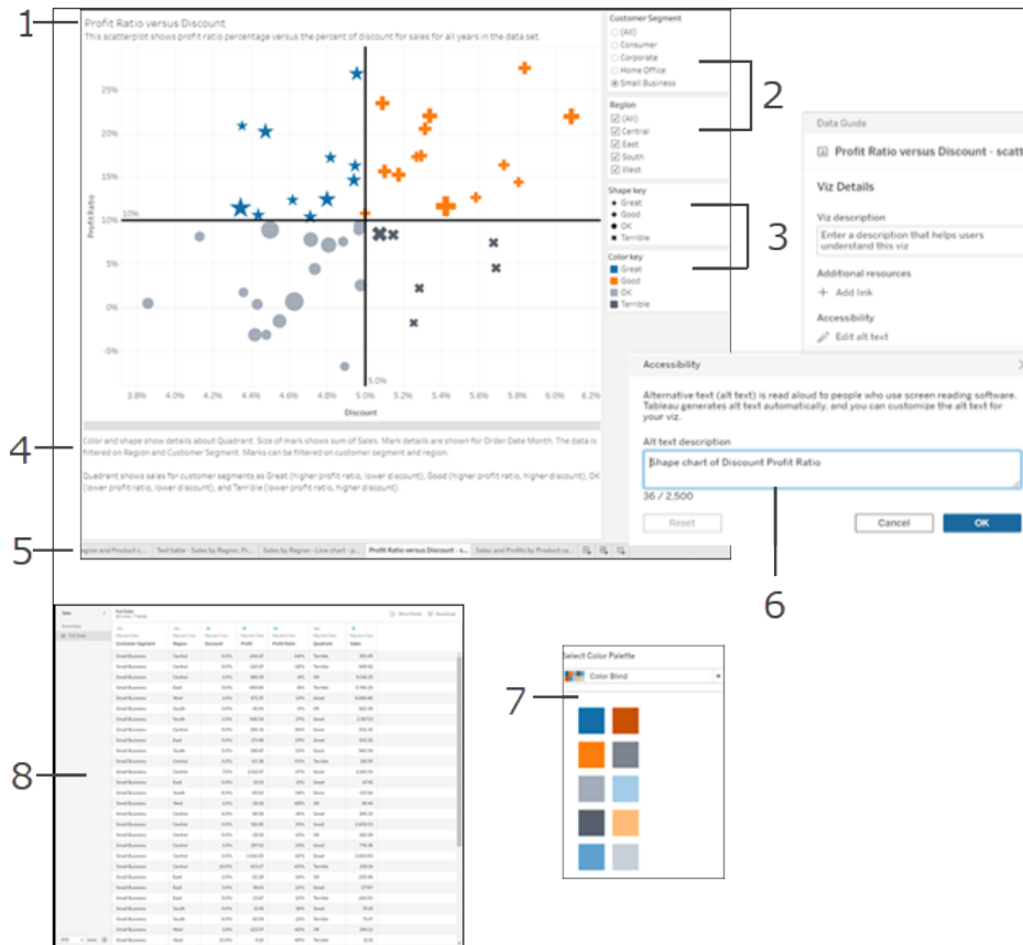
Title (1), single and multi-value filters (2), categorical legends (3), captions (4), tabs (5), alt text for vizzes (6), Color Blind palette (7), View Data window (8).
