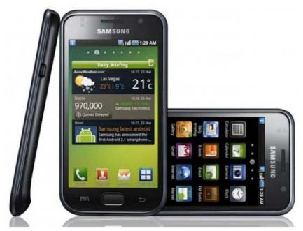
There's also A-GPS, Bluetooth 3.0, USB 2.0 and WiFi b/g/n, while onboard storage will be either 8GB or 16GB. That can be expanded courtesy of a microSD card slot happy with up to 32GB cards. Connectivity includes quadband GSM and triband (900/1900/2100) UMTS/HSPA.
