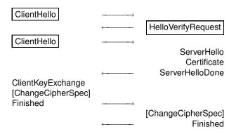
Figure 4. The simple DTLS RSA handshake
