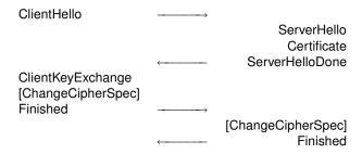
Figure 2. The simple RSA TLS handshake
