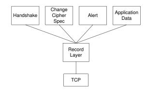
Figure 1. The Structure of TLS
