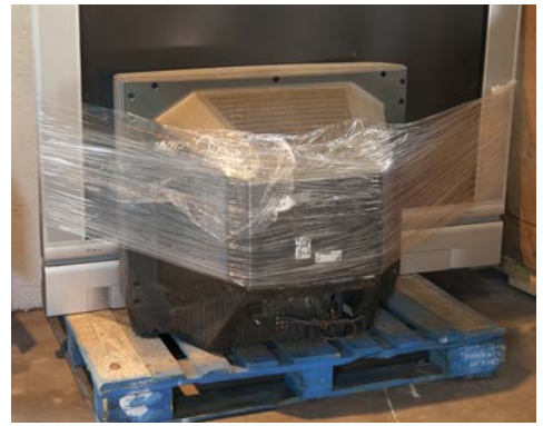
CRT TVs stacked on a pallet with screens facing inward and secured with shrink wrap.
